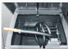
Electric fuel refilling pump
