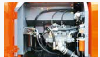
Grouped remote filters and inspection points
